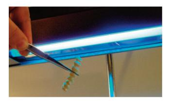
Checking Zirconia prostheses after sintering avoids to proceed in manufacturing in presence of cracks
